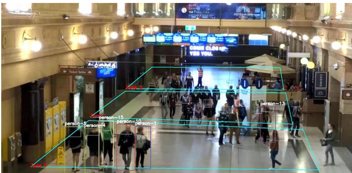
Figure 9 Camera feed analysis – annotated and anonymized video with the overlay of the zones of interest
